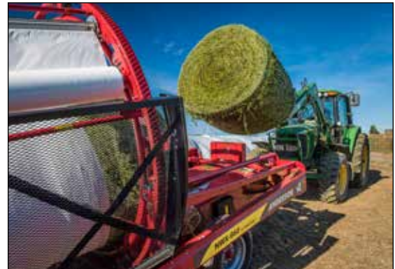
Figure 2-30. Making haylage by wrapping high moisture round bales in UV-resistant stretch wrap allows the harvest of quality forage and helps avoid rain damage.
